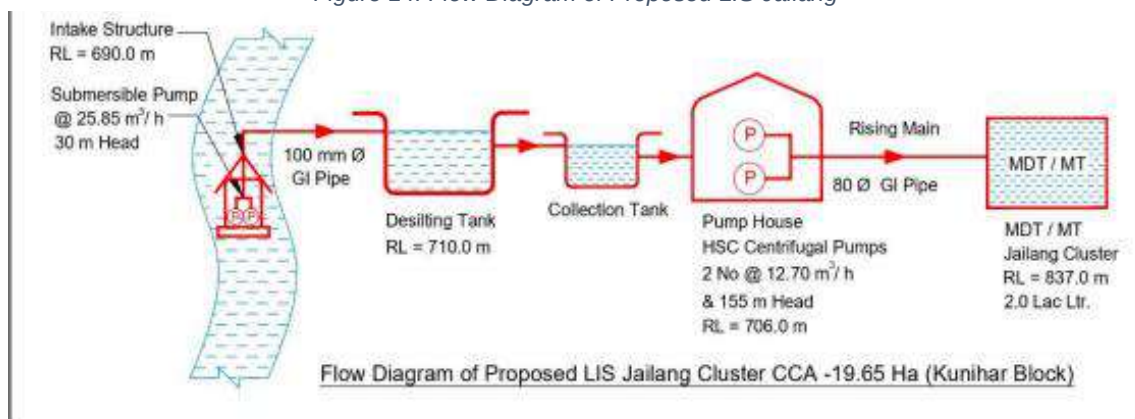
Figure 14: Flow Diagram of Proposed LIS Jailang
