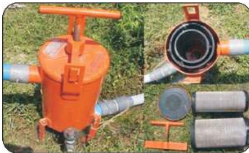
Fig.1.3 Screen filter showing steel wire mesh strainers
