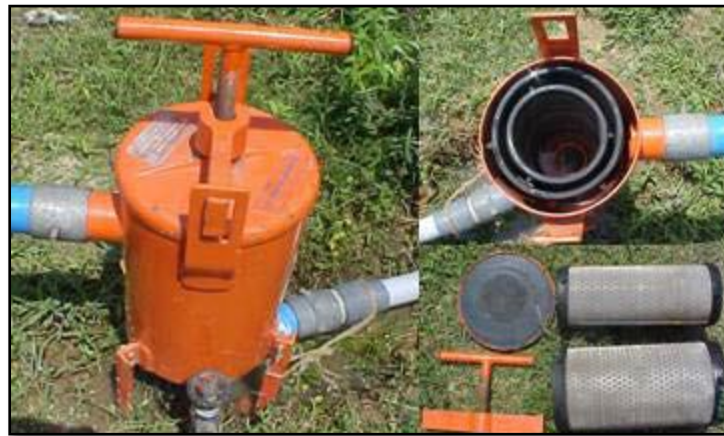
Fig.1.3 Screen filter showing steel wire mesh strainers
